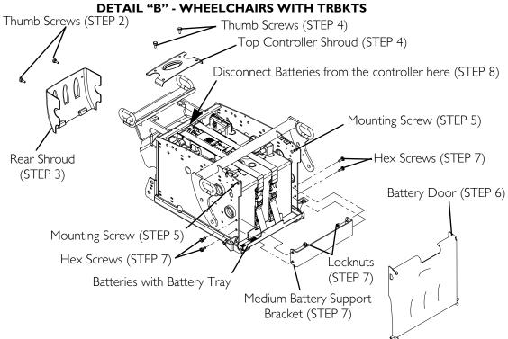
FIGURE 10.2 Removing the Battery Door and Rear Shrouds
